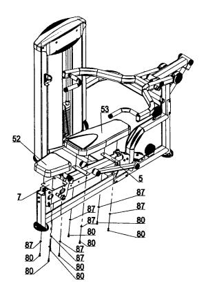
Fix back cushion(53) to back adjusting tube(5), using 4 hex head bolt M10x25(80) and 4 flat washers(87). Install the seat cushion(52) to the seat adjusting tube(7) using 4 hex head bolt M10x25(80) and 4 flat washers(87). Using right tools tighten bolts and nuts properly.
