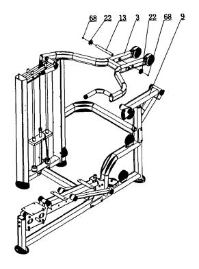
Assemble arm frame(3) to adjustable frame(9) using pivot shaft(13), 2 ending cap(22) and 2 flat head Allen bolt M8x15(68). Using the right tools to tighten bolts and nuts properly.
