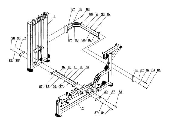
Assemble the tower frame(1) to the main frame(2) using lower connect tube(10) and upper connect tube(4). Fix it to fixing plate(38), fixing plate(39), and using 4 pan head Allen bolt M10x125(84), 2 pan head Allen bolt M10x100(83), 2 pan head Allen bolt M10x25(80), 14 flat washer(87), 2 spring washer(88). Adjust the position of the equipment, and then using the right tools tighten bolts and nuts properly.
