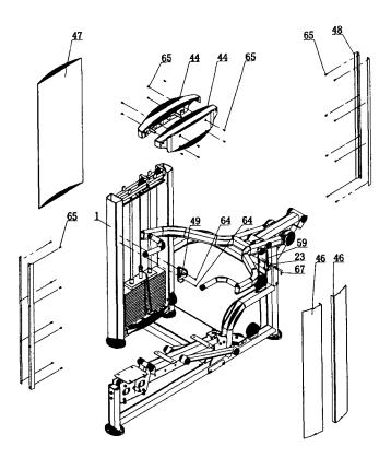
Fix 4 side faces(48) in the tower frame(1) using pan head Phillips bolt M6x15(65), 8 in the front and 8 in the back, using the right tools tighten bolts properly. Insert 2 front covers (46) and 1 back cover(47) in the tower frame(1). Then fix the bottle cage (49) on the tower frame(1), using pan head Phillips bolt M5x15(64), and using the right tools tighten bolts properly. Put top cover(44) on the tower frame(1).
