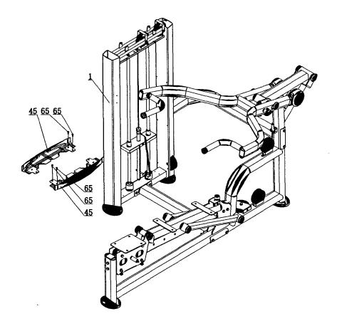
Fix2 base cover(45) to tower frame(1) using 4 panhead Phillips bolt M6x15(65). Using right tools tighten bolts properly.
